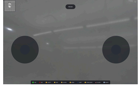
Fig. 3: Web-based teleoperation interface for Reachy Mini. The operator streams live camera footage while controlling the robot via a mobile device, where physical phone orientation maps directly to the robot’s head pose, creating an intuitive first-person embodiment analogous to a VR system.
