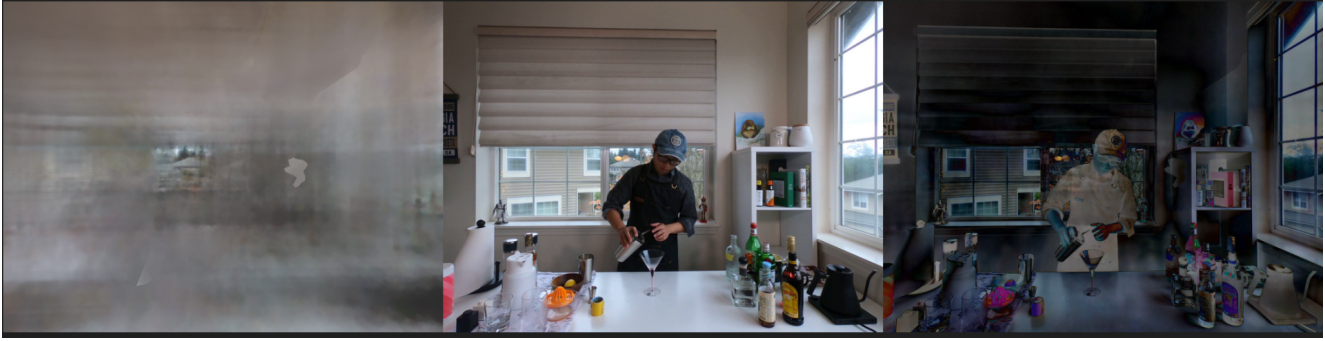
Figure 4. Effects of SSIM Loss. (left) the generated test image. (middle) the ground-truth test image. (right) the error map between the generated image and the ground-truth image, which was calculated using an L1 distance metric. The model reconstructed the entire scene uniformly.
